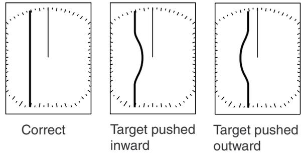
*Improper and correct sweep timing*
