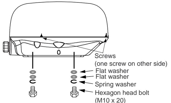
*Antenna unit, showing location of mounting hardware*
